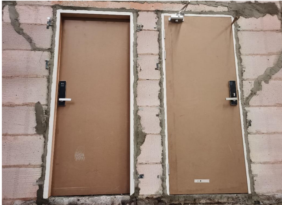
Fig. 1 Exposed Side Prior to the Fire Test
