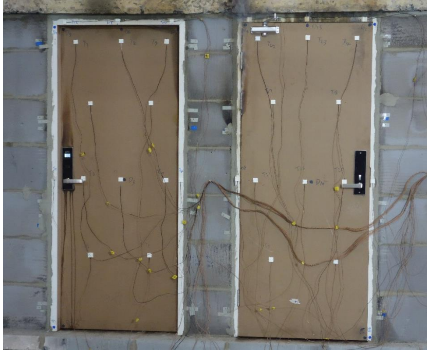
Fig. 3 Unexposed Side after 20 Minutes
