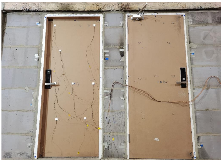
Fig. 2 Unexposed Side Prior to the Fire Test
