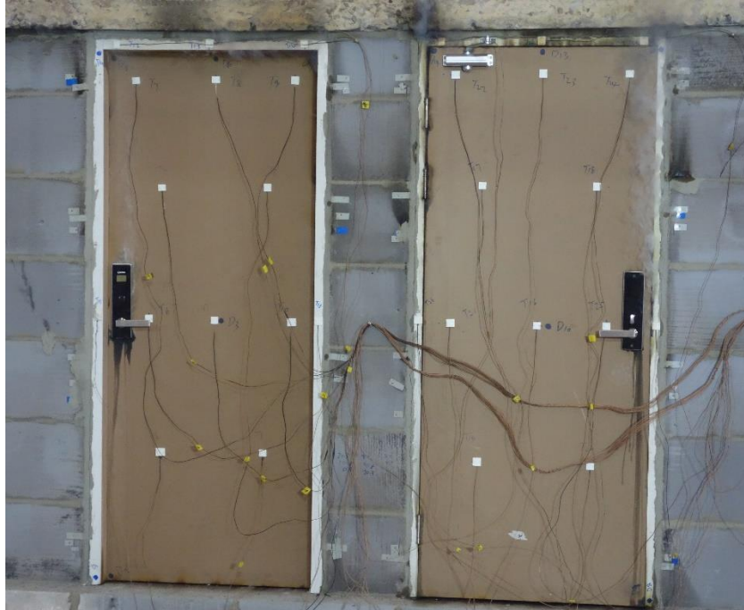
Fig. 5 Unexposed Side after 68 Minutes
