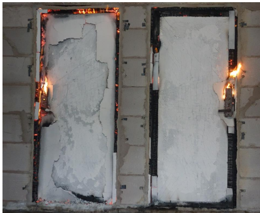
Fig. 6 Exposed Side after 68 Minutes
